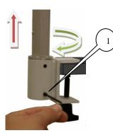
The threaded hole at the foot of the support arm must match the lower threaded hole of the clamping device.
